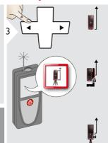
Distance is measured from the rear of the device (standard setting).
