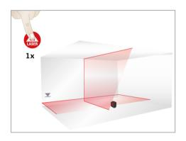
Vertical lines and horizontal lines on
