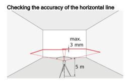
Place the lock switch in the "Unlocked" position (see Levelling lock). Position the instrument approx. 5 m away from the wall. Direct the instrument at the wall and switch on. Activate the laser line and mark the intersection point of laser crosshairs on the wall. Swivel the instrument to the right and then to the left. Observe the vertical deviation of the horizontal line from the marking. If the difference does not exceed 3 mm, then the instrument is within tolerance.
