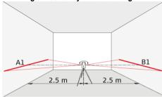
Set the instrument on a tripod half-way between two walls (A+B) that are approx. 5 m apart. Place the lock switch in the "Unlocked" position (see Levelling lock). Direct the instrument at wall A and switch on the instrument. Activate the horizontal laser line or laser point and mark the position of the line or the point on wall (A1). Rotate the instrument by 180° and mark the horizontal laser line or the laser point in exactly the same way on wall (B1).
