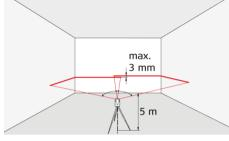
Place the lock switch in the "Unlocked" position (see Levelling lock). Position the instrument approx. 5 m away from the wall. Direct the instrument at the wall and switch on. Activate the laser line and mark the intersection point of laser crosshairs on the wall. Swivel the instrument to the right and then to the left. Observe the vertical deviation of the horizontal line from the marking. If the difference does not exceed 3 mm, then the instrument is within tolerance.
