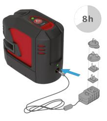
Charge the Li-Ion battery before using it for the first time. While charging, the instrument may heat up. This is normal and should not affect the instrument's lifespan or performance. At the recommended storage temperature of  $-20^{\circ}$ C to  $+30^{\circ}$ C ( $-4^{\circ}$ F to  $+86^{\circ}$ F), batteries containing a 50% to 100% charge can be stored up to 1 year. After this storage period the batteries must be recharged.
