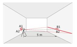
Then place the instrument at the same elevation as close as possible to wall A and again mark the horizontal laser line or the laser point on wall A (A2). Rotate the instrument by  $180^{\circ}$  again and mark the laser on wall B (B2). Measure the distances of the marked points A1-A2 and B1-B2. Calculate the difference of the two measurements.
