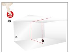
Vertical line and dots on
