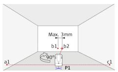
Then rotate the device exactly 90° clockwise around the plumb point P1 and position the left-
