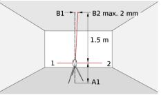
Place the lock switch in the "Unlocked" position (see Levelling lock). Set up the laser on its tripod to wall mount bracket near point A1 at a minimum distance of 1.5 m from point B1. The horizontal laser is aligned in direction 1. Mark the laser points A1 and B1 with a pin.
