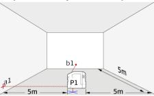
Place lock switch in "Unlocked" position (see Levelling lock). Mark a reference point (P1) approx. 5m from the walls and position the lower plumb point exactly on it. Align the cross hair to the left wall and mark the intersection point (a1) approx. on the same hight like P1 to the wall. Shortly after mark the right-hand perpendicular beam (b1) on the front wall.
