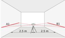
Set the instrument on a tripod half-way between two walls (A+B) that are approx. 5 m apart. Place the lock switch in the "Unlocked" position (see Levelling lock). Direct the instrument at wall A and switch on the instrument. Activate the horizontal laser line or laser point and mark the position of the line or the point on wall (A1). Rotate the instrument by 180° and mark the horizontal laser line or the laser point in exactly the same way on wall (B1).
