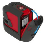
Insert the battery-pack by pressing it down and then tilting it towards the housing as shown until it snaps in.
