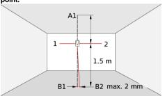
Rotate the instrument by 180° so that it points in the opposite direction 2 to direction 1. Adjust the instrument so that the laser beam hits point A1 exactly. If point B2 is no further than 2 mm away from point B1, then the instrument is within tolerance.
