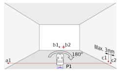
Afterwards turn the device exactly 180° around the plumb point P1 and position the right-hand perpendicular beam to the existing reference point a1. Make sure that the upper plumb point is still exactly on the reference P1. Then mark the left-hand beam to the right wall and mark it with c2. Finally measure the difference between the former reference point c1 and the new point c2. The deviation may be max. 3mm between these two points.
